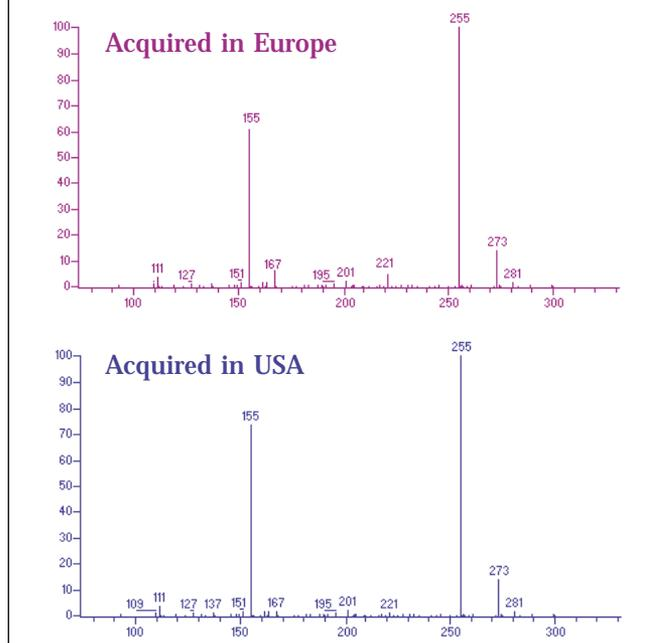
MS/MS spectra acquired from two different instruments, one in Europe the other in the USA. These spectra show the power of *Normalized Collision Energy* to create reproducible spectra suitable for databases and libraries.
