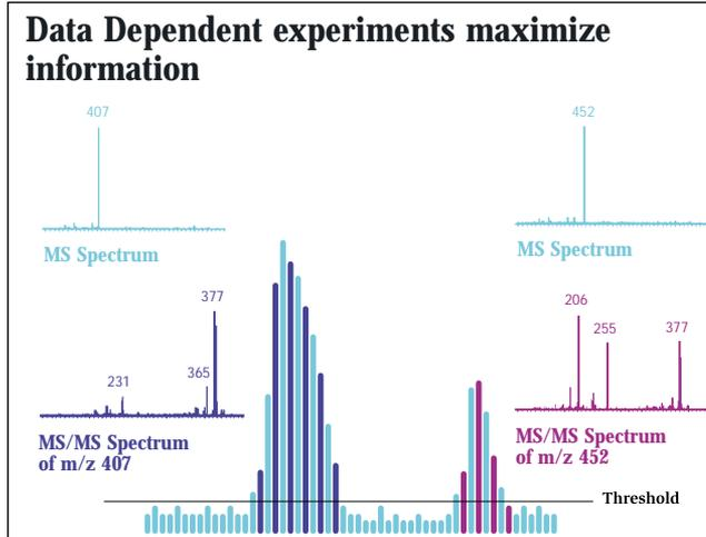
*Data Dependent MS and MS/MS generate the maximum amount of information from a single run.*
