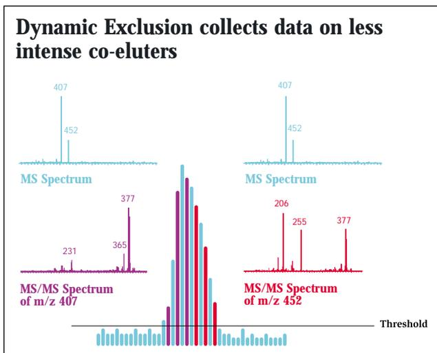
*Two compounds with molecular ions at  $m/z$  407 and  $m/z$  452 co-elute. Using Dynamic Exclusion, after MS/MS scans of  $m/z$  407 have been acquired, the ion is placed on the exclusion list and MS/MS spectra of the minor component at  $m/z$  452 are collected.*
