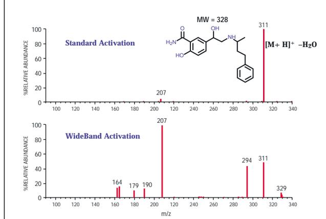
MS/MS spectra of labetalol acquired with and without *WideBand Activation*. Standard activation conditions, even with high collision energy, show only the water loss ion. In contrast, *WideBand Activation* generates extensive and meaningful fragmentation data in qualitative applications.
