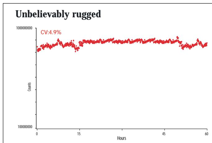
*Analysis of reserpine in 10 mM sodium phosphate buffer. Data shows over 1000 injections in 60 hours with no decrease in signal.*
