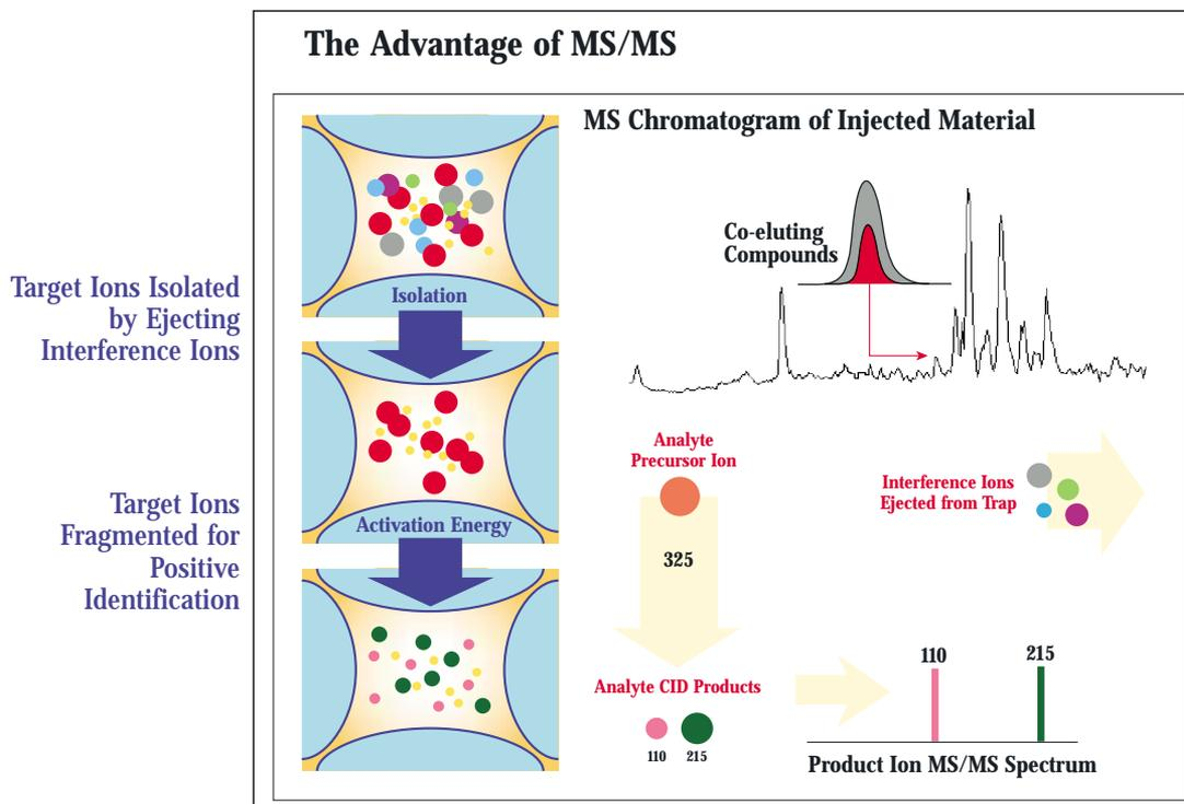
MS/MS provides product ion spectra, which quantify and distinguish analytes in complex matrices. This process is accomplished automatically in an HPLC experiment on the LCQ Advantage.
