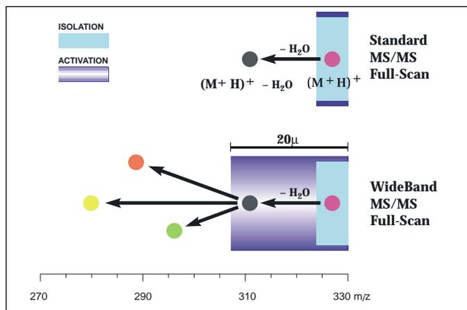
*WideBand Activation* applies resonance energy over a mass range that extends 20µ lower than the selected ion.
